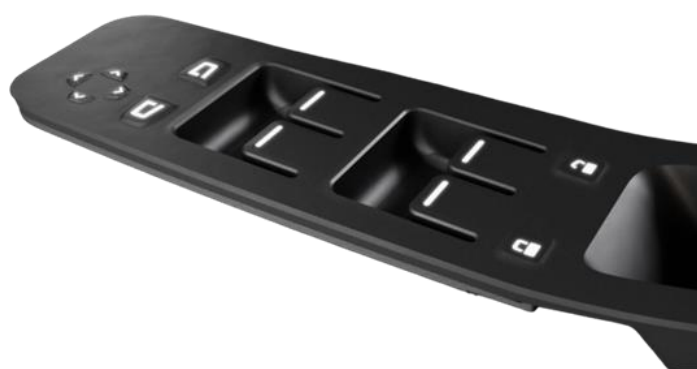
Window lifter controller using active Plastic technology (source: Novares & TG0)
