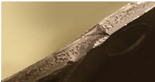
Detail of plastic part injected with blowing agent (source: Novares)
